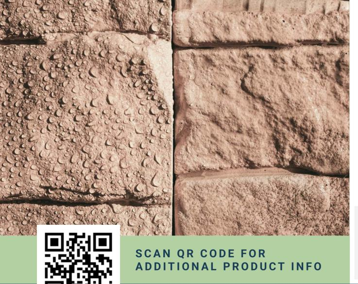
**SPRAY**: Saturate from bottom up. Apply enough for a 4-8in rundown below the spray contact point. Let first application penetrate for 5-10 min before applying second coat. NOTE: When spraying fluted architectural block, spray in an overlapping X-pattern. Wipe up any excess material using microfiber cloths.
